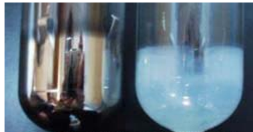
Left Tube = Vacuum Present Right Tube = Faulty
